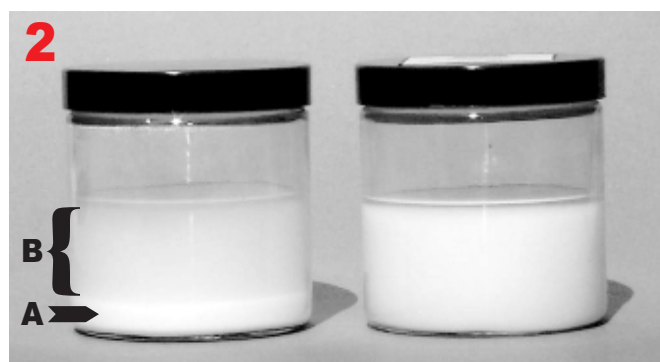
2. After seven minutes, the micropowder (left) shows significant band of solids, settling (arrow A) out of the carrying agent. The remaining mixture is smoothly graduated, ranging from nearly clear (at the top) to a more concentrated mix immediately at the bottom (bracket B). These variations make smooth, even lubrication difficult.
