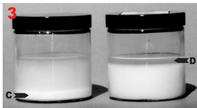
3. After 20 minutes, the micropowder has settled almost completely (C) and will need significant agitation to return to a mixed state. Meanwhile, below a small layer of carrying agent (right, D), the rest of the VCG mix remains an even, consistent suspension.
