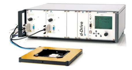
flexure system create a completely play free motion. Overshooting (oscillation) is actively minimized by controllable setting and resetting forces (generated by two different actuating systems). Even under full load pre-selected positions can be reached in milliseconds with nanometer accuracy. This is an essential characteristic especially for high-speed scanning.
